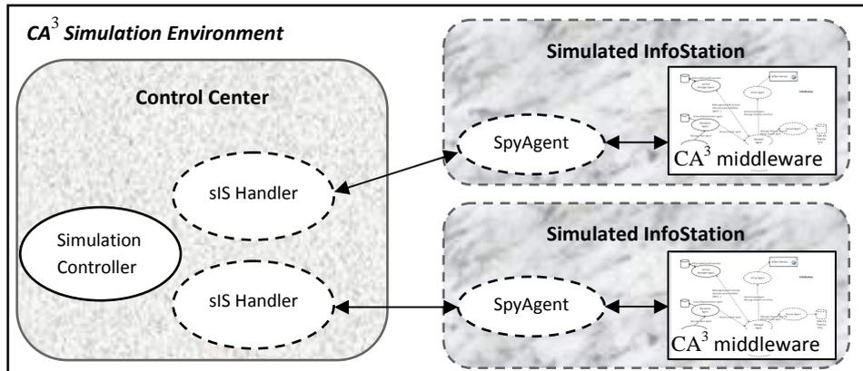
**Fig. 2** CA<sup>3</sup> Simulation Environment
