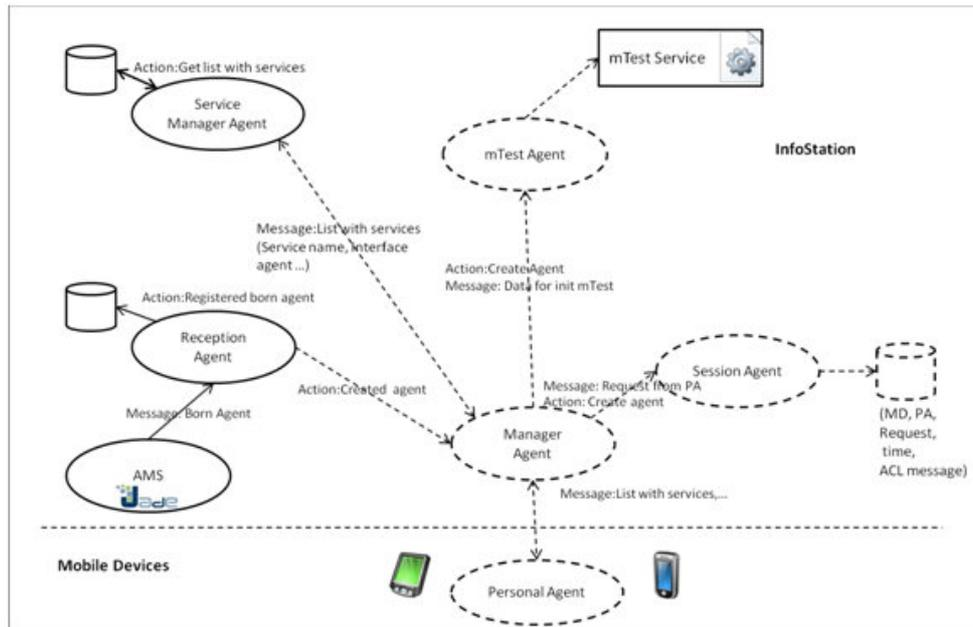
**Fig.1.** The WiFi-based middleware InfoStation's architecture
